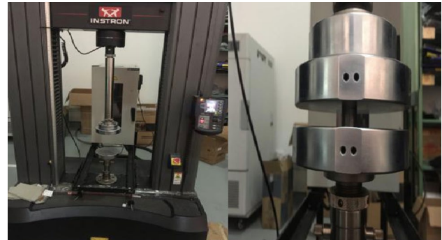
Fig. 6 Foam aluminum composite structure on test machine
