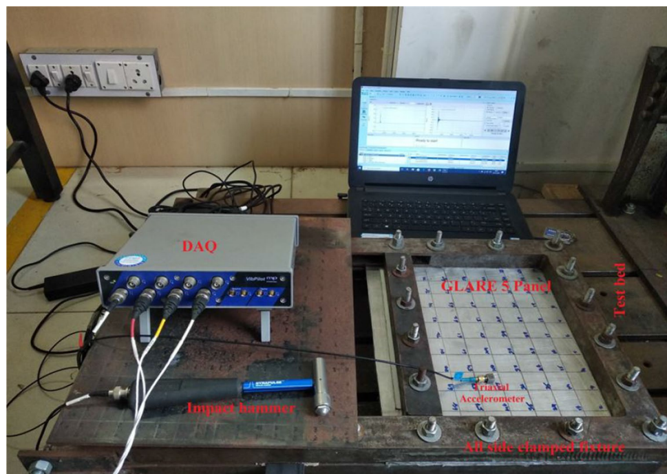
Fig. 8 Experimental test setup for free vibration of GLARE-5 panel for all side clamped boundary condition
