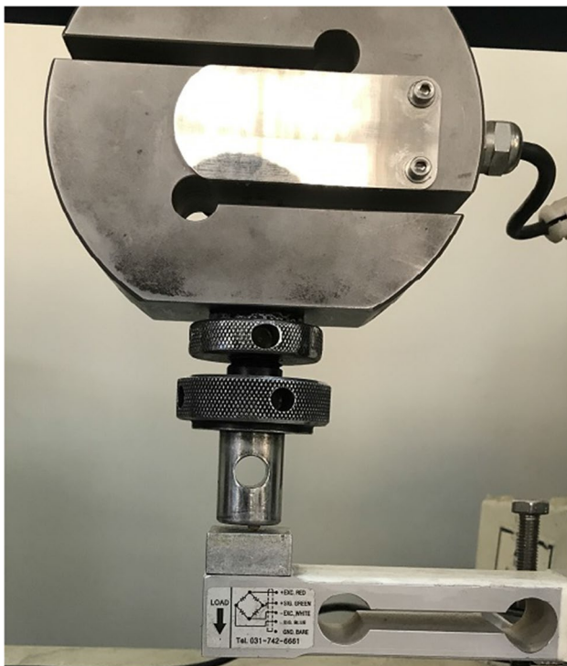
Fig. 1 Articular cartilage sample under unconfined stress-relaxation test
