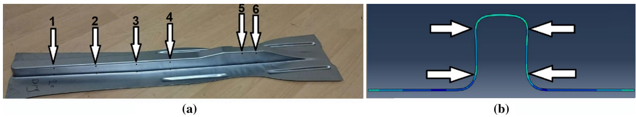
Fig. 12 Positions of measuring points on drawn walls at 6 locations a experiment b finite element model
