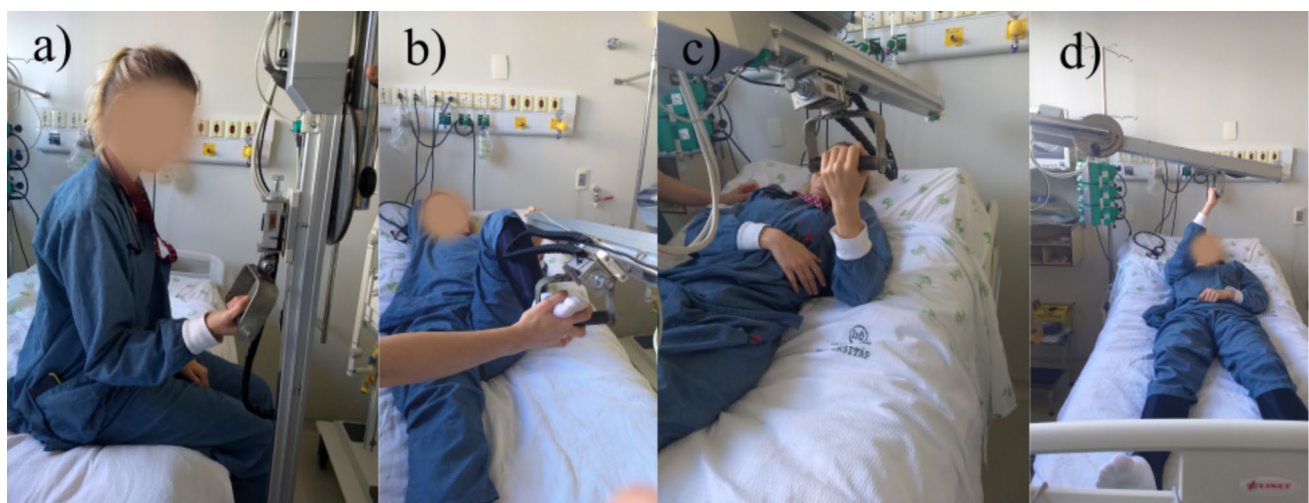
Fig. 14 Different training configuration in SARPA: a and c elbow flexion/extension, b hip and knee flexion/extension, and d shoulder adduction
