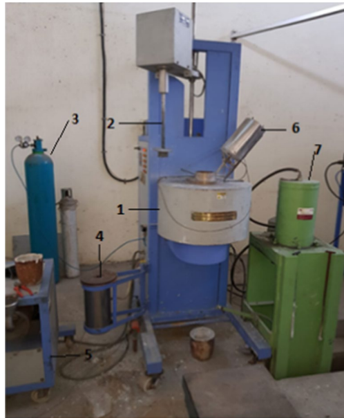
1.Furnace 2. Mechanical stirrer 3. Argon gas cylinder 4. Vacuum die 5. Centrifugal cast setup 6.Powder heater 7. Squeeze cast setup
