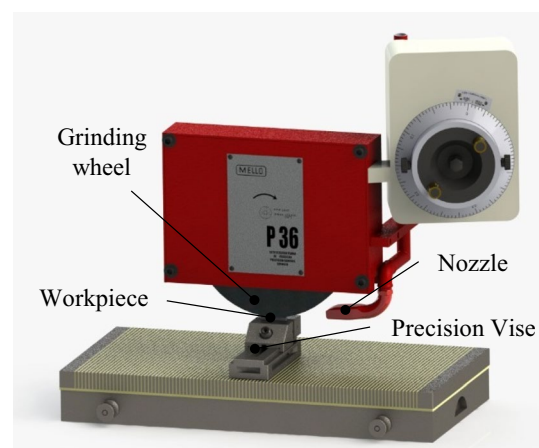
Fig. 2 Schematic illustration of the setup used for the grinding experiments
