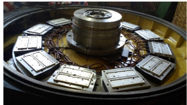
Fig. 16 Oil pad tilting static pressure bearing
