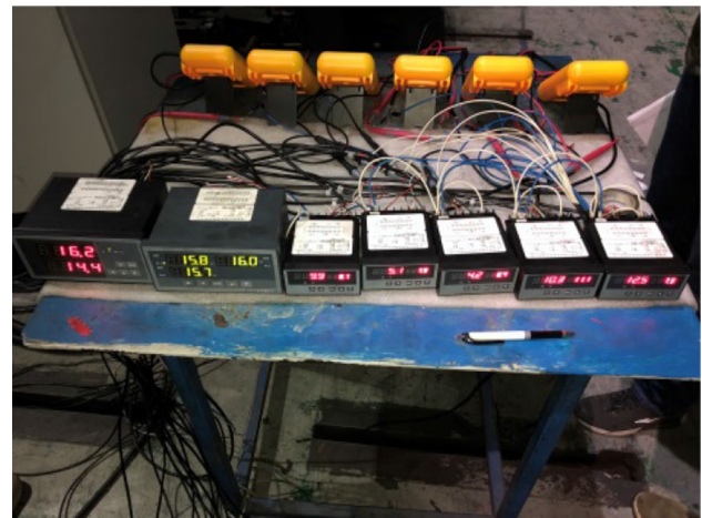
Fig. 21 Data acquisition and display system
