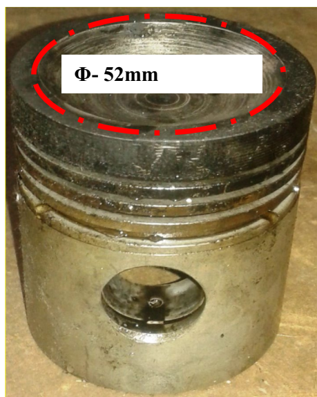
Fig. 4 Hemispherical piston bowl
