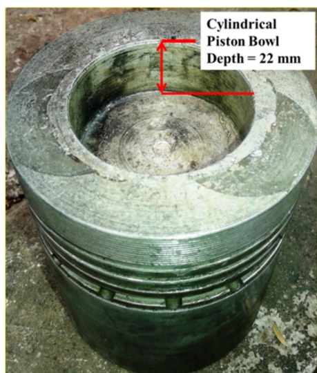
Fig. 5 Cylindrical piston bowl
