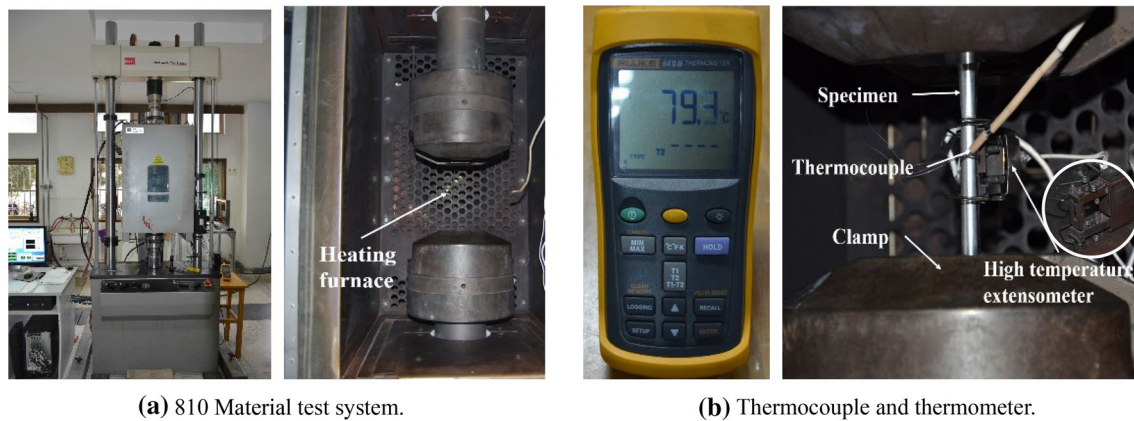
Fig. 1 Experimental apparatus at the temperature range of 25–500 °C. a 810 material test system. b Thermocouple and thermometer
