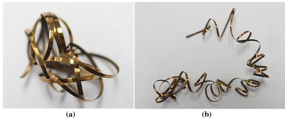
Fig. 4 Aggregation of chips. a Dry machining, b LN 2 machining
