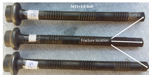
Fig. 1 Photograph of the broken down three bolts at the threads
