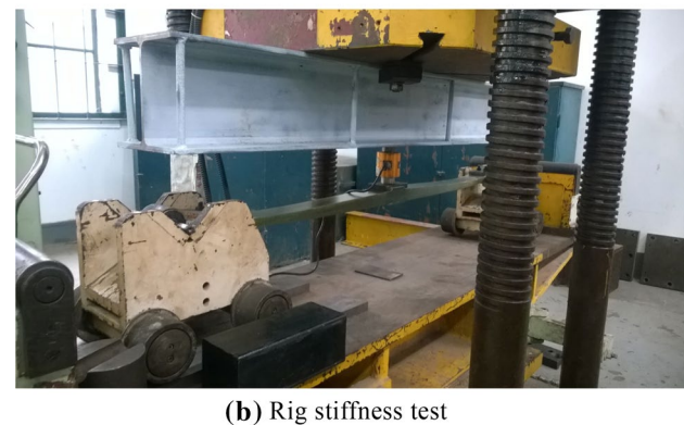
Fig. 3 Finite element simulation and rig stiffness test of the composite mono leaf spring [2]
