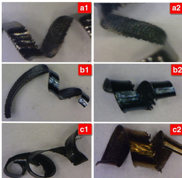
Fig. 9 Chip morphology when textured insert was applied at different depths of cut ( a1–a2 ) without any lubricant ( b1–b2 ) with graphite powder impregnation ( c1–c2 ) with MQL application for doc of 0.5 mm and 1 mm, respectively
