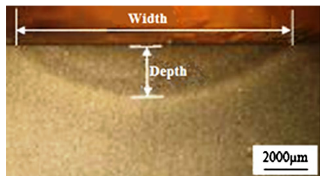
Fig. 1 Specimen cross-section and geometrical responses of the hardened zone
