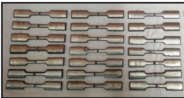
Fig. 3 Sample tensile specimens extracted from the tubes
