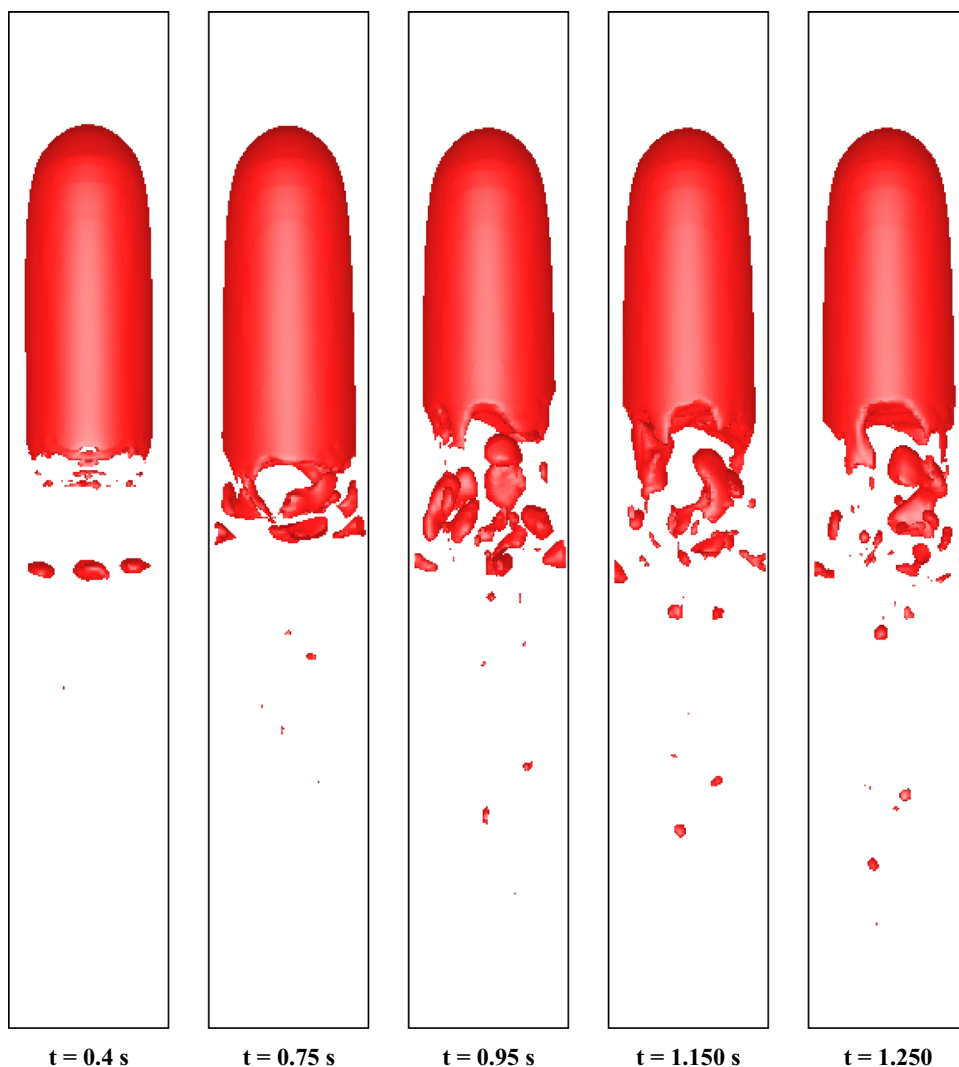
Fig. 8 Temporal evolution of Taylor bubble shape in 0.1 wt% CMC solution
