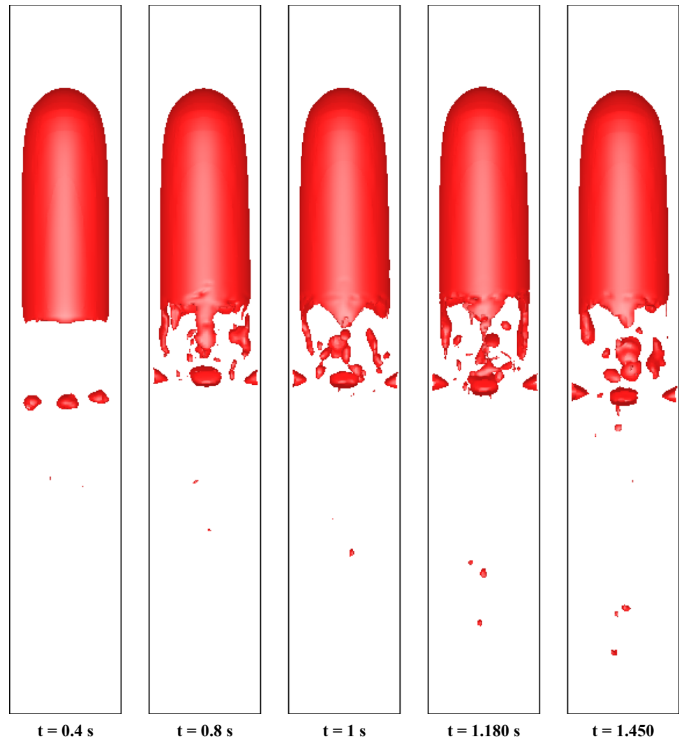
Fig. 9 Temporal evolution of Taylor bubble shape in 0.3 wt% CMC solution
