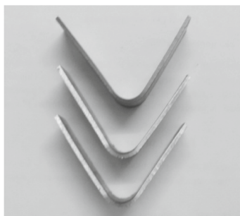
Fig 7.17 Punch radius 6mm, die opening 20mm and sheet thickness 1.5mm
