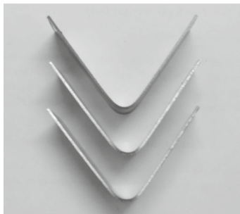
Fig 7.14 Punch radius 4mm, die opening 20mm and sheet thickness 1.0mm
