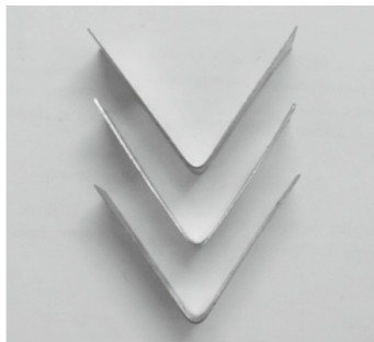
Fig 7.11 Punch radius 2mm, die opening 20mm and sheet thickness 0.5mm
