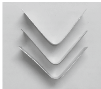
Fig 7.16 Punch radius 4mm, die opening 40mm and sheet thickness 0.5mm
