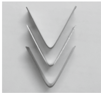
Fig 7.12 Punch radius 2mm, die opening 30mm and sheet thickness 1.0mm
