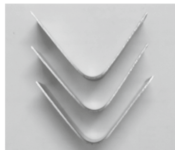
Fig 7.19 Punch radius 6mm, die opening 40mm and sheet thickness 1.0mm
