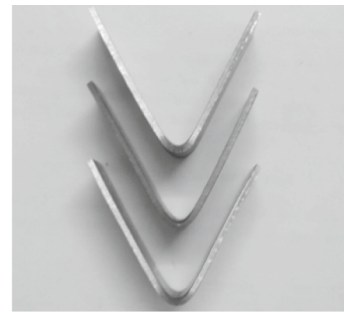
Fig 7.13 Punch radius 2mm, die opening 40mm and sheet thickness 1.5mm
