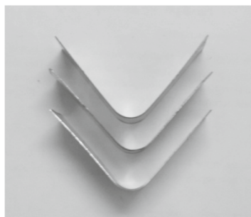
Fig 7.18 Punch radius 6mm, die opening 30mm and sheet thickness 0.5mm
