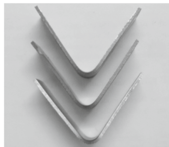
Fig 7.15 Punch radius 4mm, die opening 30mm and sheet thickness 1.5mm
