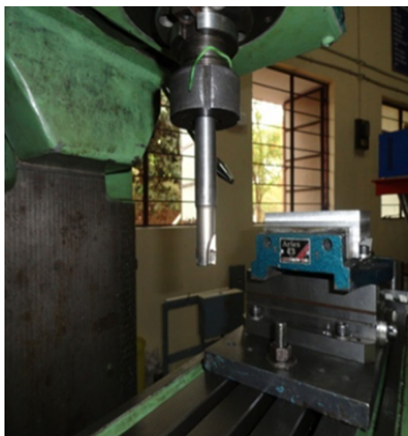
Fig. 3 BFW universal milling machine
