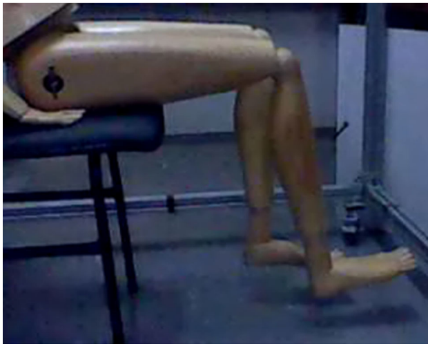
Fig. 5 Knee flexion/extension experimental test with one cable
