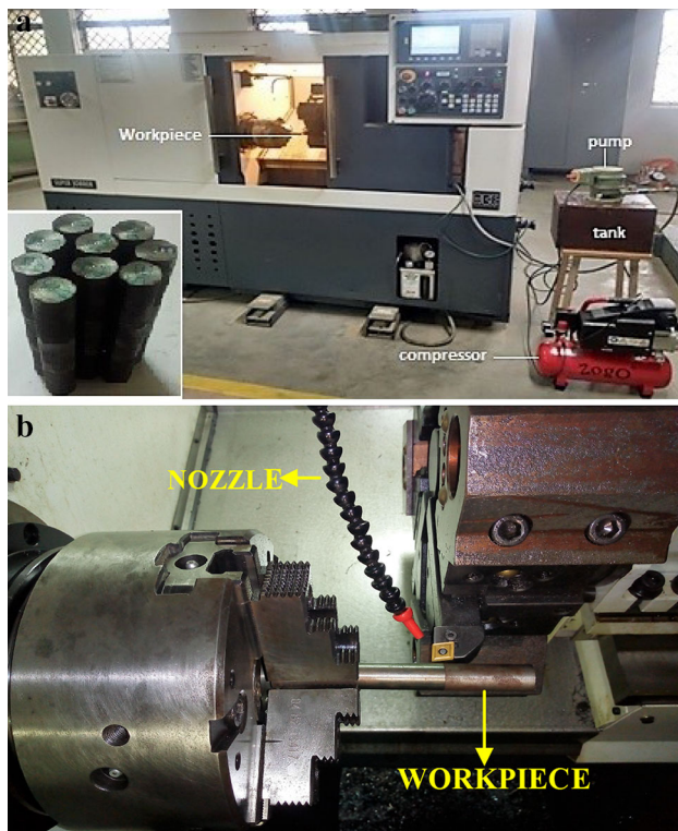
Fig. 3 a CNC machining centre. b Enlarged view of machining area
