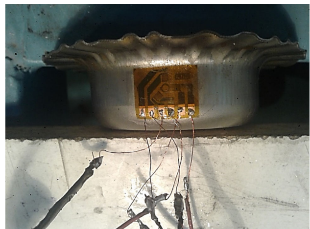
Fig. 3 Rosette strain gage attached to the cup
