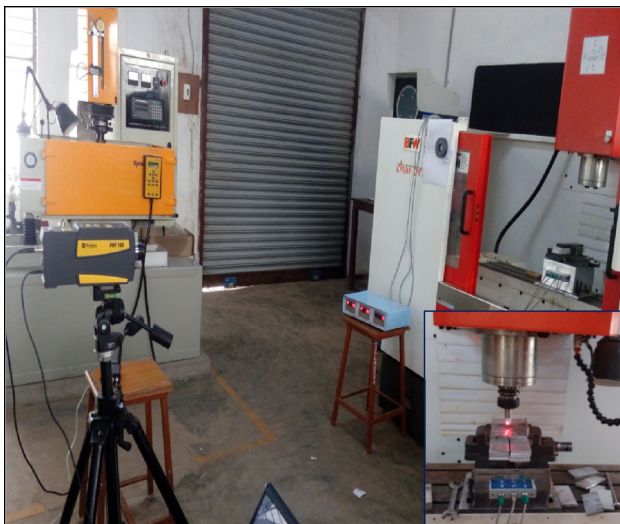
Fig. 2 Experimental setup for friction stir welding
