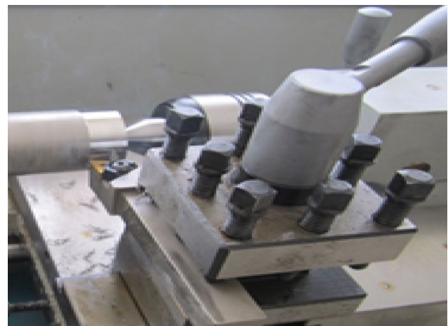
Fig. 1 Turning of Ti-6Al-4V alloy
