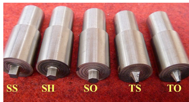
Fig. 1 Different tool geometries utilized; SS straight square, TS tapered square, SH straight hexagon, SO straight octagon, TO tapered octagon
