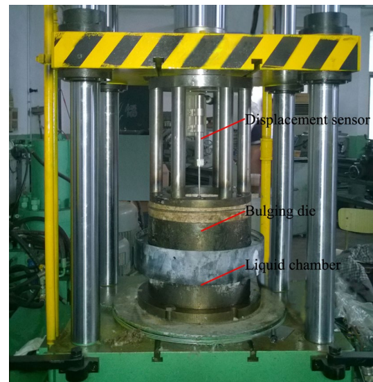
Fig. 3 Equipment of hydraulic bulging test
