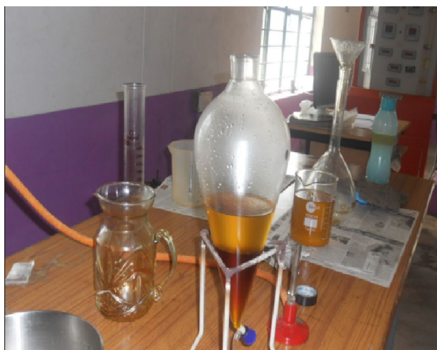
Fig. 1 Transesterification set-up for biodiesel production
