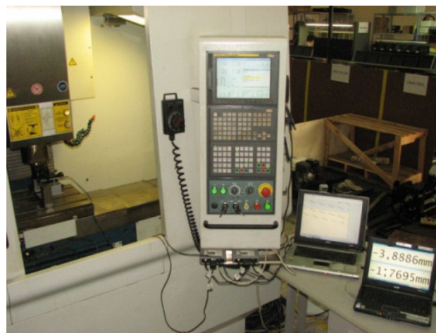
Fig. 2 The ROMI discovery 560 CNC machining center, its FANUC 20i CNC control and measurement arrangement
