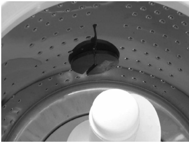
Fig. 4 Unbalance load mounted in the inner surface of the basket
