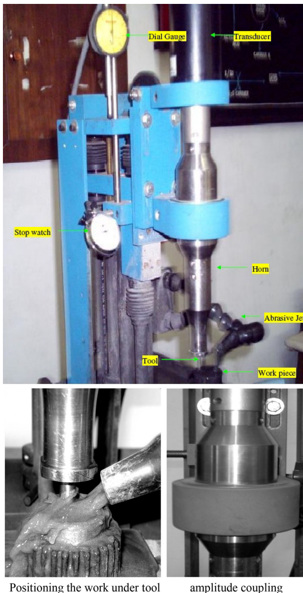
Fig. 2 Detailed representation of USM apparatus used
