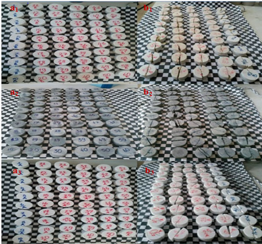
Fig. 8 Brazilian tensile strength samples views. a1, b1. natural (dry) samples, a2, b2. samples after the thermal shock cycles, a3, b3 samples after the thermal ageing cycles. a1: MB, a2: YB, a3: AB
