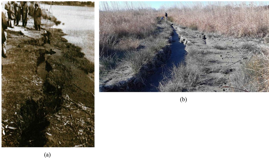
Fig. 14 Examples of lateral earth spread: a along Buna river bank, 1979; b along Erzeni river bank, 2019
