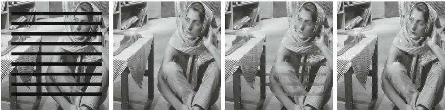
Fig. 10 Left to right: image to be inpainted, inpainting results of TV - H^{-1} , TV - L^2 and our model
