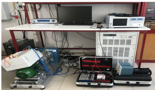
Fig. 8 Test rig with the current probe, acquisition board, loading system, and induction motor (Color figure online)
