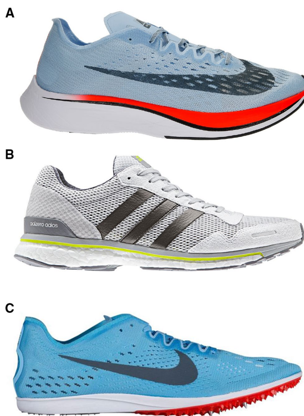
Fig. 1 The three racing shoe models used in this study. a The NVF midsole comprises ZoomX foam made with polyether block amide, an embedded carbon-fiber plate, 31 mm heel height, and 21 mm forefoot height; b ADI midsole comprises BOOST foam made with thermoplastic polyurethane, 23 mm heel height, and 13 mm forefoot height; c NZM midsole comprises Cushlon foam made with ethylene-vinyl acetate, and a plastic horseshoe spike plate with four 6.35 mm stainless steel spikes. As a fourth shoe condition, we also added 30–35 g of lead weights to the NVF (NVF+) to equalize to the greater mass of the ADI shoes to examine the confounding effects of shoe mass on the energetic cost of running. NVF Nike Zoom Vaporfly 4%, ADI Adidas Adios BOOST 3, NZM Nike Zoom Matumbo 3
