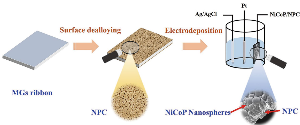
Fig. 17 Schematic illustration of the preparation of the NiCoP/NP Cu nanocomposite. Reprinted with permission from [59]
