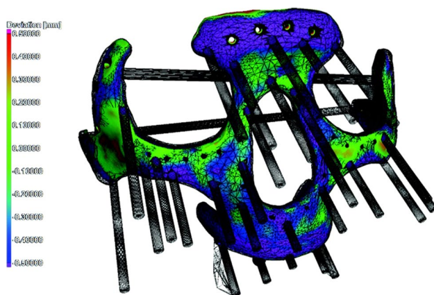
Fig. 7 CAD variance analysis of facial implant built by LPBF [9]
