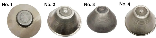
Fig. 4 Oblique views of AZ31B sheets after hot shear spinning (373 K, 473 K, 573 K and 673 K)
