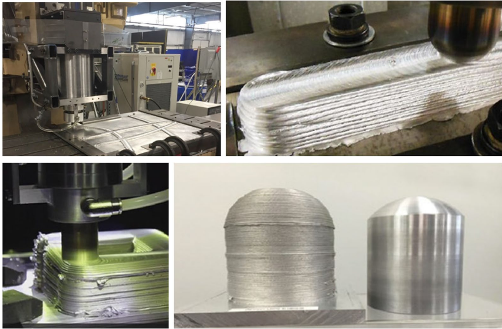
Fig. 7 Products fabricated by using FSP additive manufacturing technology of the MELD manufacturing company [132]
