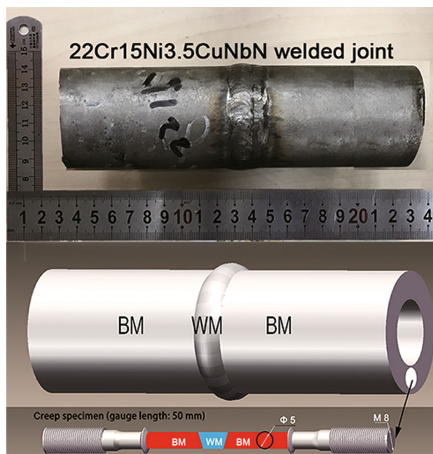
Fig. 1 22Cr15Ni3.5CuNbN weldment and the schematic representation of the sampling location for creep strain tests
