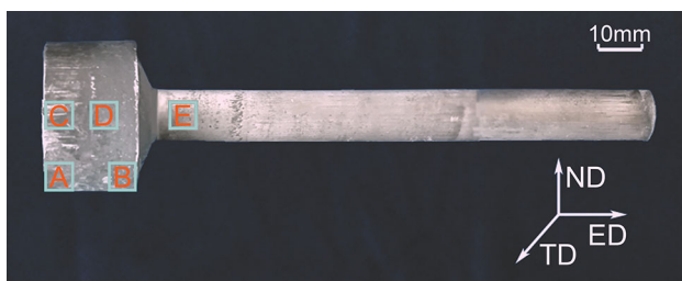
Fig. 2 Interrupted extrudate with five characteristic locations labeled A, B, C, D, and E
