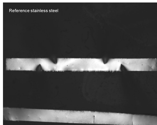
Fig. 7 Micrograph of the 4-needle setup in one reference stainless steel stripe. The width of the stripes is 800 μm
