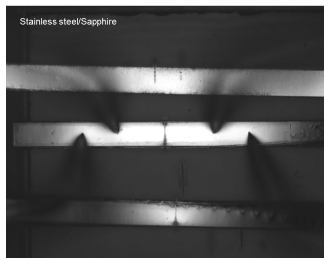
Fig. 8 Micrograph of the 4-needle setup in one of the laser-welded stainless steel stripes with sapphire. The width of the stripes is 800 μm
