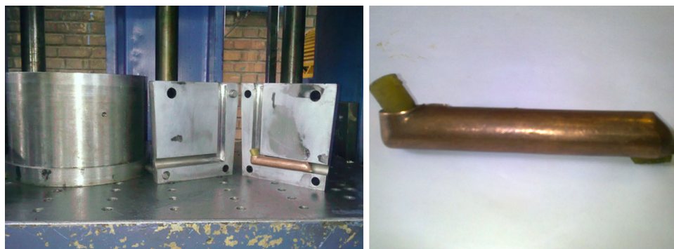
Fig. 3 ECAP die set up with the rubber pad sample and formed work piece after one pass ECAP
