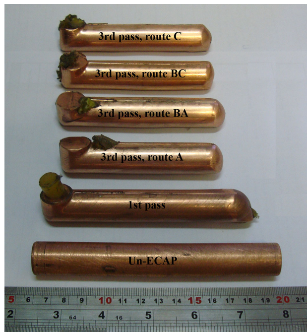
Fig. 5 CP Cu tube samples before and after ECAP process using routes A, B A , B C , and C
