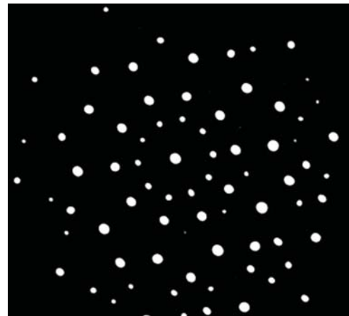
Fig. 9 Selected area diffraction pattern with 5-fold symmetry from rapidly solidified \text{Mg}_{32}(\text{Al, Zn})_{49} [24]
