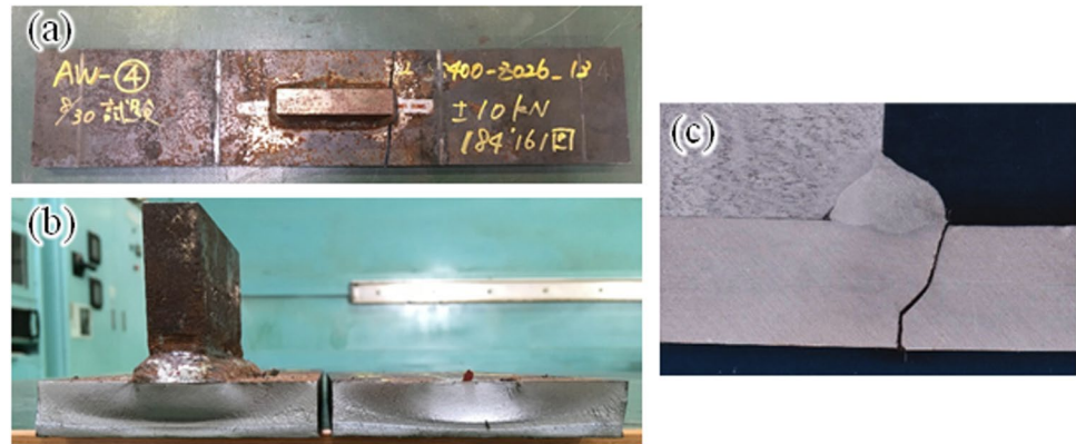
Fig. 12 GW specimen after fatigue test (a appearance, b fracture surface, c crack propagation path)
