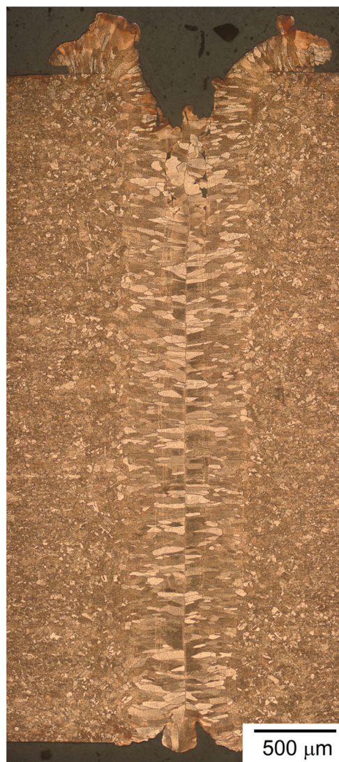
Fig. 15 Light optical micrograph of an etched cross section of a weld generated with v = 530 \text{ mm s}^{-1}
