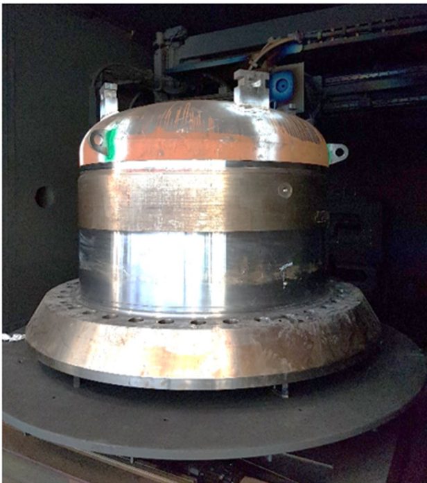
Fig. 2 Mock-up component to be welded including a shell-to-head weld and impingement (not visible) installed on the turn table. Electron beam gun in background. Head installed using lifting lugs
