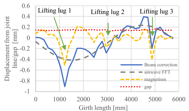
Fig. 11 Result of the seam tracking with post-processing
