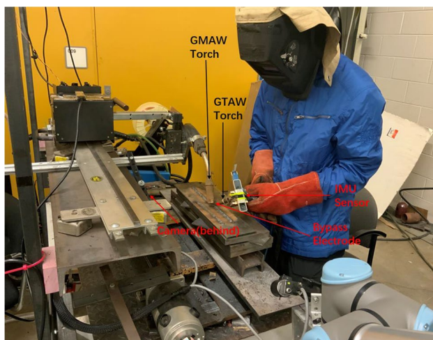
Fig. 2 Experimental setup. The power sources are not shown
