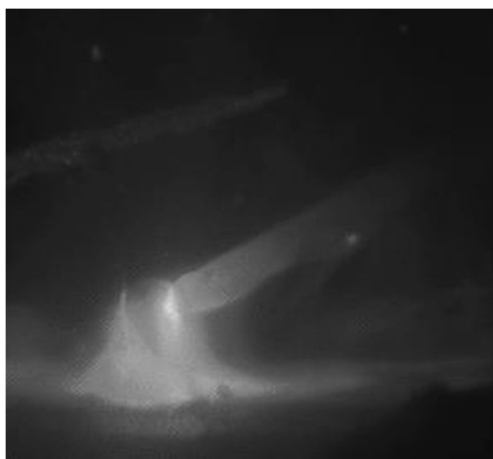
Fig. 18 Examples of the mixed mode in DE-GMAW
