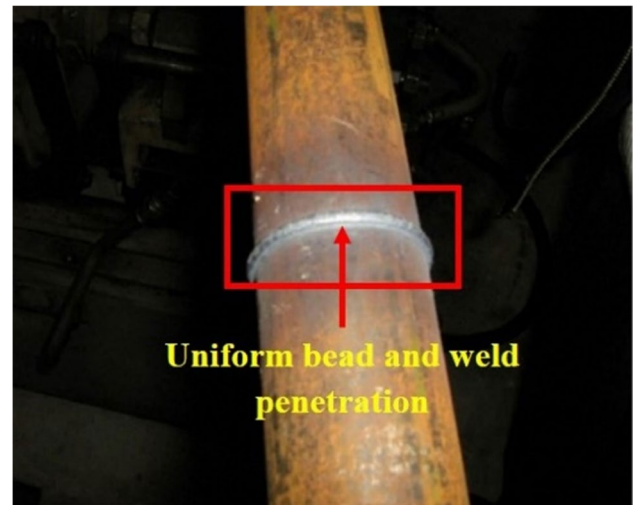
Fig. 9 Uniform bead and weld penetration of MIAB-welded T11 tubes [6]
