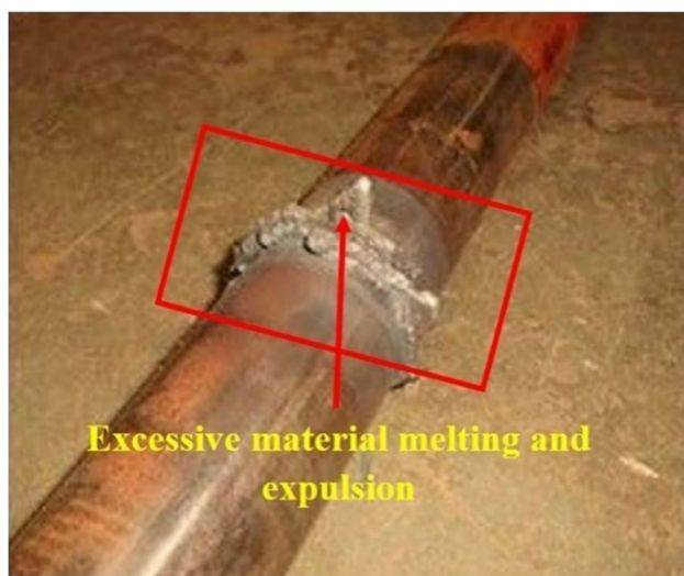
Fig. 15 MIAB-welded T11 joint with excessive metal expulsion [7]
