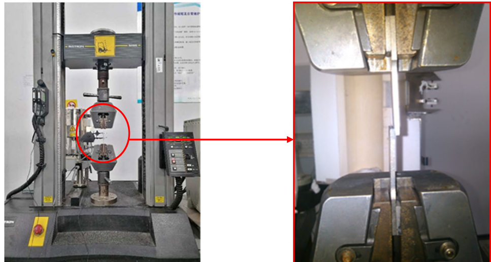
Fig. 3 INSTRON 5869 material testing machine
